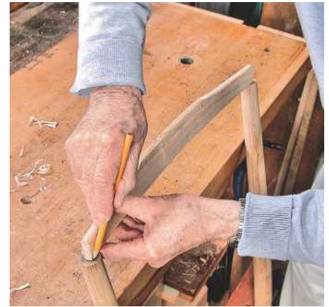
▲ Pic. 4 Using the rail's end as a templet to locate the mortise
